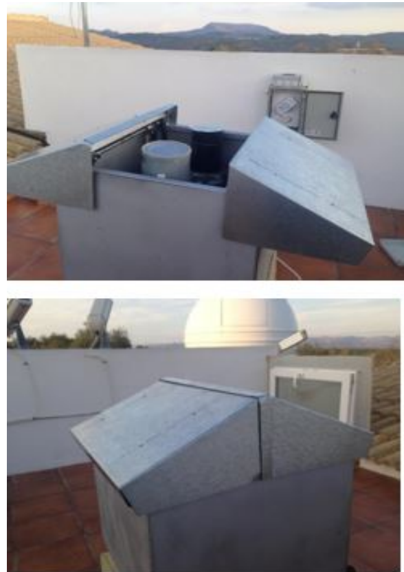
Fig. 2. Autonomous Mini Observatory operating with the two spectrographs inside.
