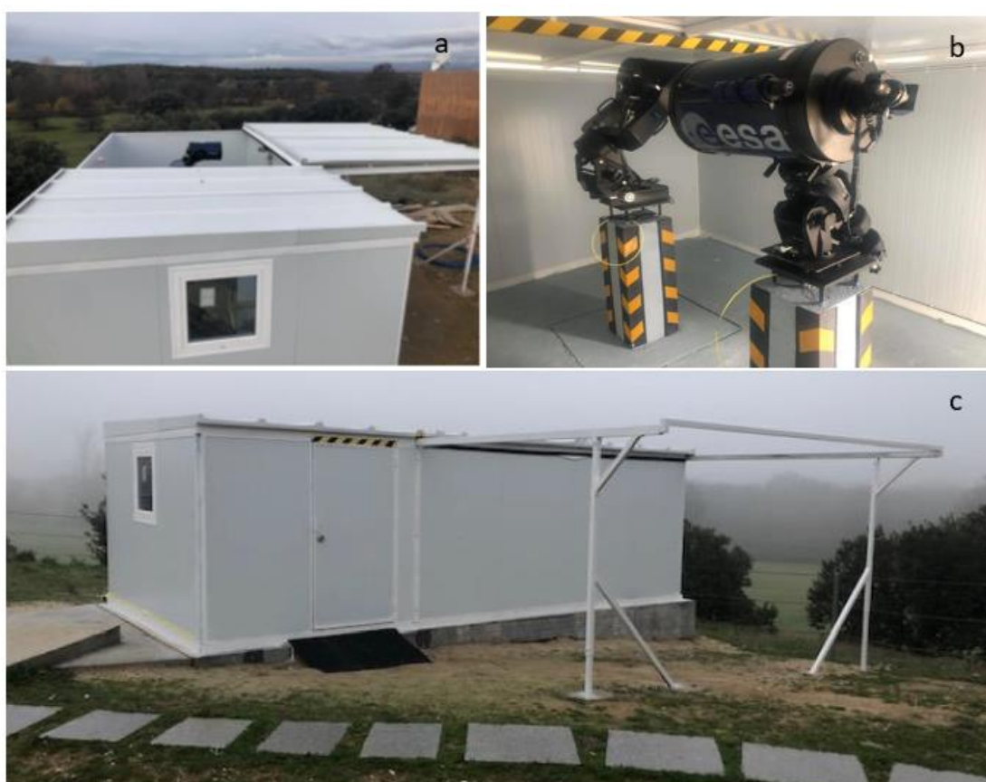
Figure 2. CESAR Astronomical Observatory. ESA-ESAC (Villafranca del Castillo-Madrid). RAO with open roll-off roof (a). S/C 12" telescopes (each one on one of the two pillars displayed in the picture) at f/10 and two CCD cameras, Atik 314 L+ and Atik 4400 (b). RAO with closed roll-off roof (c).
