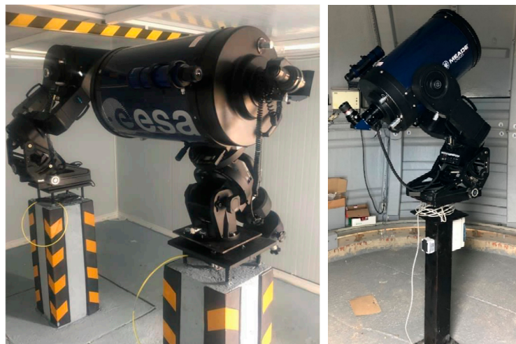
Figure 4. Schmidt–Cassegrain (S/C) telescopes on EQ8 German equatorial mounts on a support consisting of a reinforced concrete pillar anchored to the ground by an isolated footing structure ( left ). S/C telescope on a lightweight equatorial wedge and pillar with double leveling plate, made of structural steel with electrical panel and data inside ( right ).
