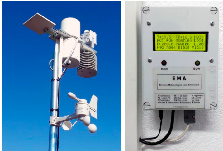
Figure 3. Weather station installed on a vertical pole ( left ). Weather station control electronics connected to a PC ( right ).
